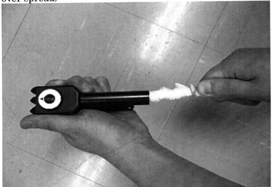
For rust proofing, apply the grease or the sewing machine oil (lubricating oil) to the cloth, and brush only the upper part of the black string chuck.
